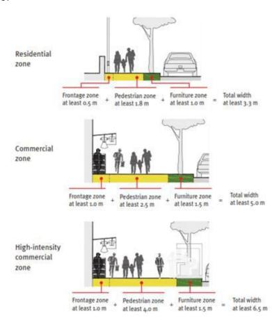
Figure 4: Minimum footpath zone dimensions for different land uses.
