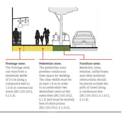
Figure 3: All footpaths must have separate zones for frontage, pedestrian movement, and furniture.
