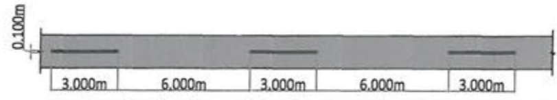
Longitudinal Marking for Signalized Junction
