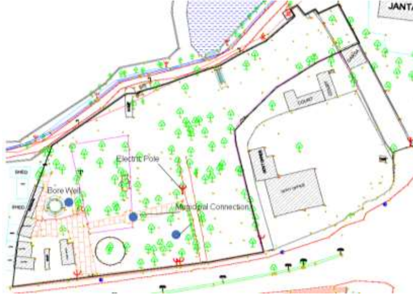
Figure – Survey Map showing existing Utilities
