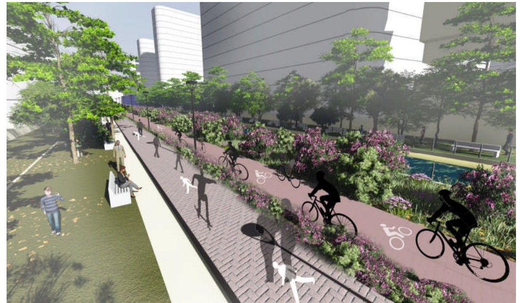
Various Linkages are provided across the development, these linkages have Activity Generating Uses at Ground Floor Level. The Walkways & Cycleways are segregated by small Green Belt to keep both separate yet together.
