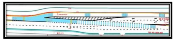
Figure 8-19 Typical Marking - weaving at the foot of the flyover
