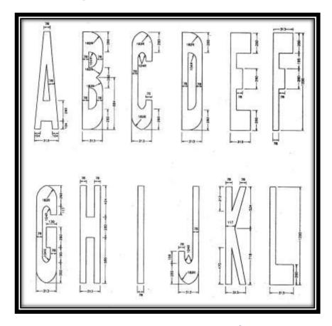
Figure 6-1 Size of the letters for word messages (speed 50 km/h or less)<sup>5</sup>
