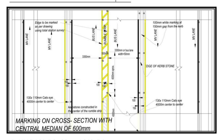
Figure 8-10 Typical longitudinal marking (centre line) on cross section for dedicated bus lanes
