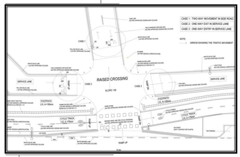
Figure 8-18: Making at raised crossings
