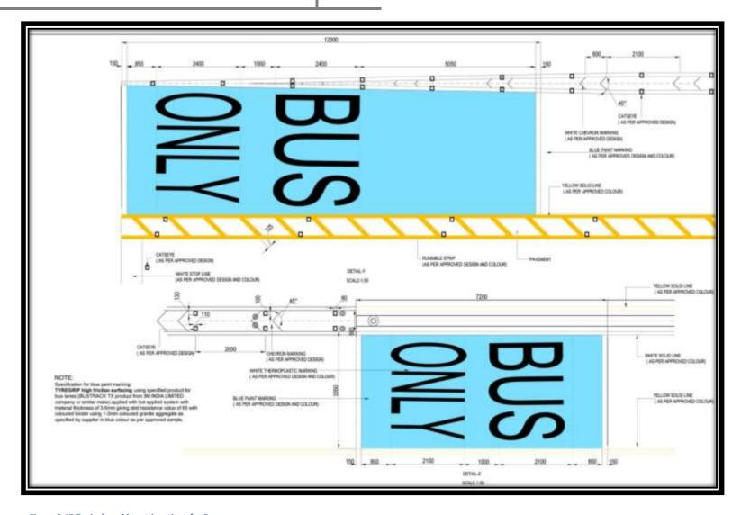
Figure 8-15 Typical marking at junctions for Buses
