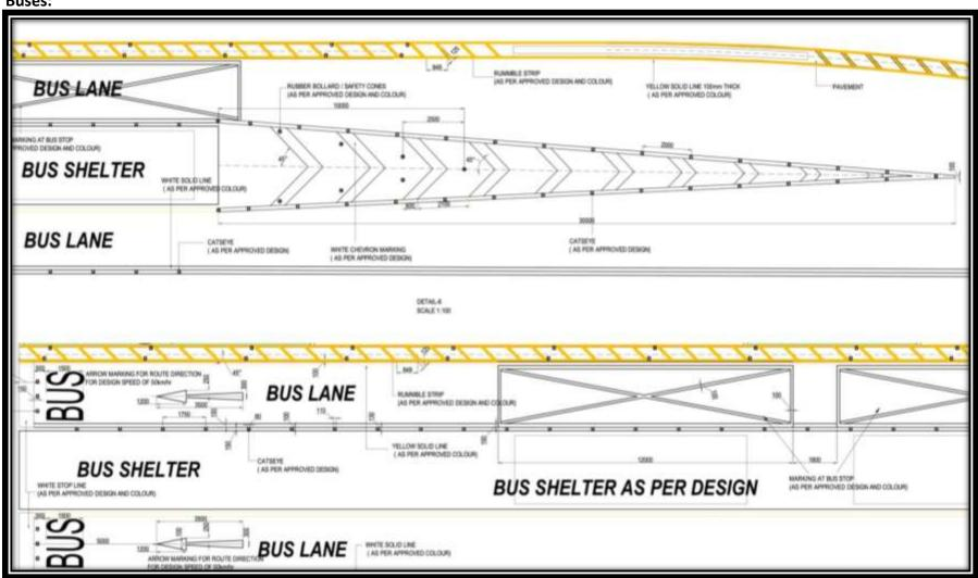
Figure 8-13: Bus marking – along the carriageway
