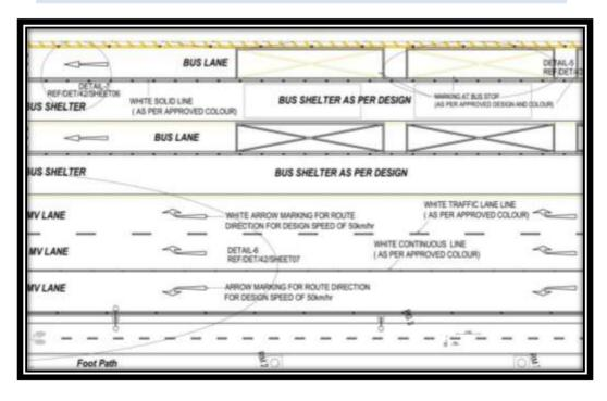
Figure 8-1: Typical marking before the junction for all road users
