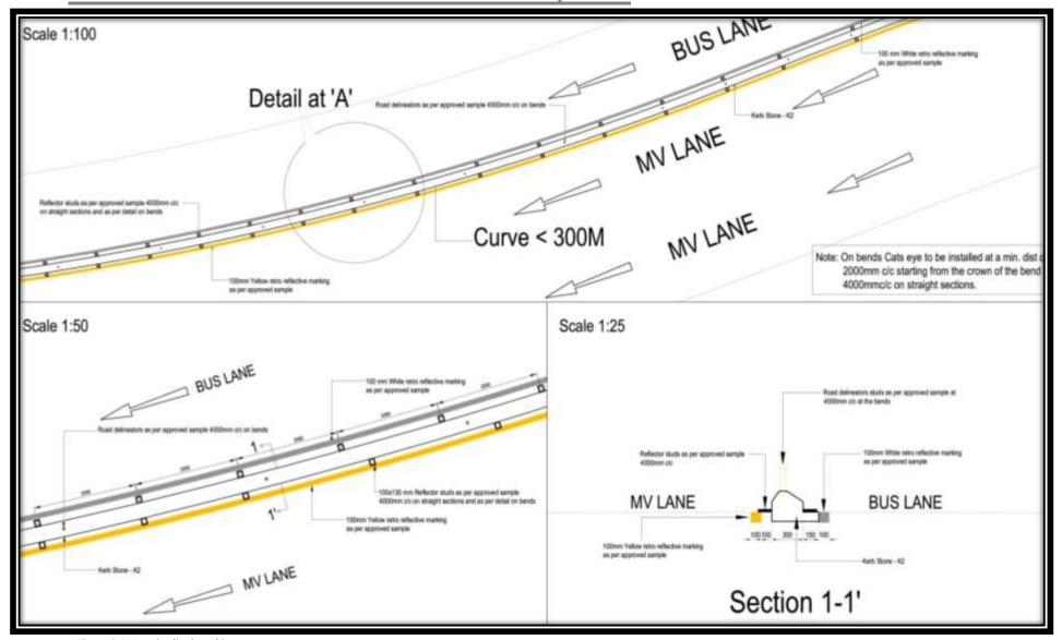
Figure 8-11 Longitudinal markings on curves
