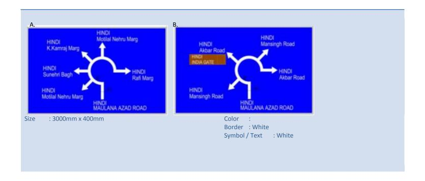
15. <u>Destination Signages</u>: Mounted on the gantries, these signs indicate the main landmark destinations.
